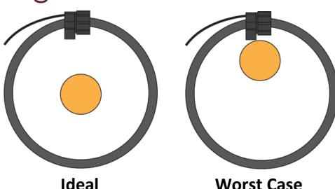
The position of the conductor inside the coil will affect the accuracy. Deviation from the centre will at worst cause a maximum of 1% deviation when the conductor is placed near the cap of the coil.
